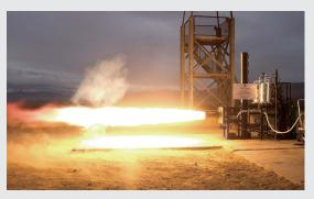
Vector rocket engine test firing
